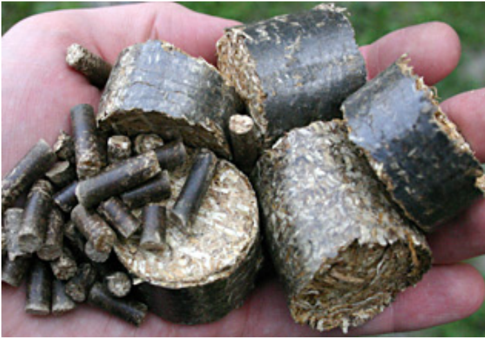
Samples of grass pellets and briquettes prepared for experimental combustion output trials.
